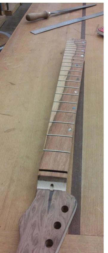
While I did a great job getting the faceplate onto the headstock, I ended up drilling a 2-½ inch long tapered trench in the middle of it for the truss rod access. So now I know to drill the access hole before gluing the faceplate.
